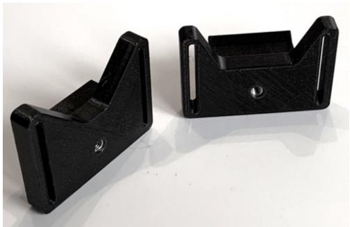
**VF prompter bracket, with an L bracket:** At the request of Rob Vouna, I made a bottom mount adapter for prompter monitors that have a ½-20 hole on the bottom.
