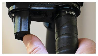
The VGTBE slides onto the Volt and snaps into place. It can also be easily removed. No tools or reworking of the Volt is required.
