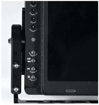
**Plain old rod mounts:** These brackets span 15mm rods on 60mm centers. One version of the mount has a 10-32 screw to fit the monitor weights. The other version has a ½-20 thread to mount other accessories. \$50 for the mount, or \$35 when bought with two weights. Shown below with a 1pound weight.
