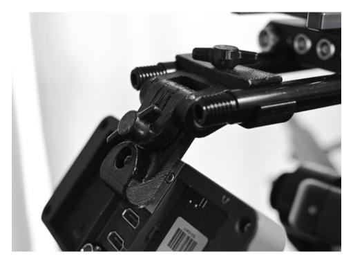
The pivoting bracket is used this way to hold a below-the-lens return monitor for talent!
