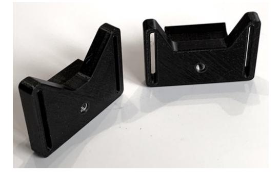
**VF prompter bracket, with an L bracket:** At the request of Rob Vouna, I made a bottom mount adapter for prompter monitors that have a <sup>1</sup>/<sub>4</sub>-20 hole on the bottom.
